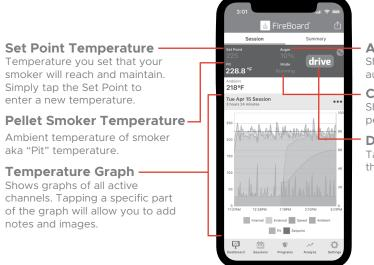
Auger Duty Cycle Shows the percentage of time the auger is spinning.
